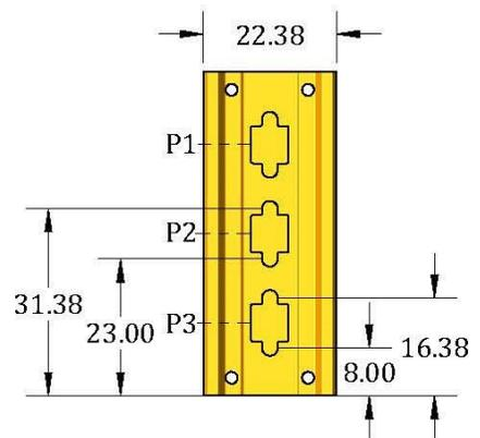
**Dimension Schemes: 4.5' Excavation Depth Configuration B - (1.38m)**
