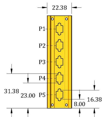
**Dimension Schemes: 7' Excavation Depth Configuration C - (2.14m)**
