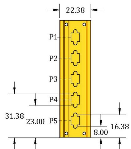
**Dimension Schemes: 7' Excavation Depth Configuration B - (2.14m)**
