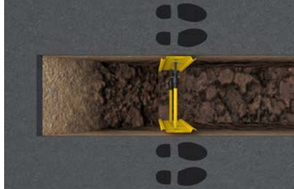
Figure 11 Operators should be a safe distance from excavation edge, ensure operatives are always in line with the assembly.
